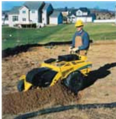
Maintenance time and cost is reduced through the use of a fully hydrostatic trencher-drive that eliminates all belts, pulleys and gears.
