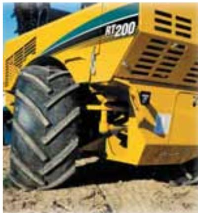
Hydrostatic ground drive and twin wheel motors eliminate the need for locking differentials while maintaining maneuverability.
